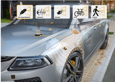
CoSSy is a sensitive sensor system for various applications to distinguish between air-borne sounds, knocking noises, dents and scratches for example.
