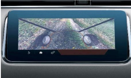
Satellite cameras make the hood transparent and give the driver a view of the ground below.
