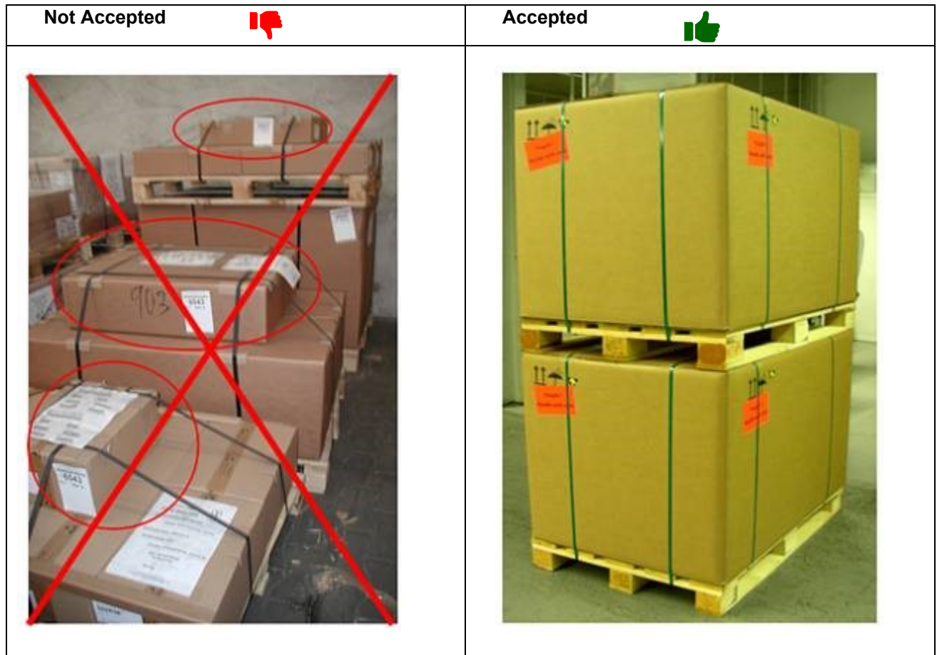
Figure 8.2-2: Not accepted and accepted loading units (LU)
