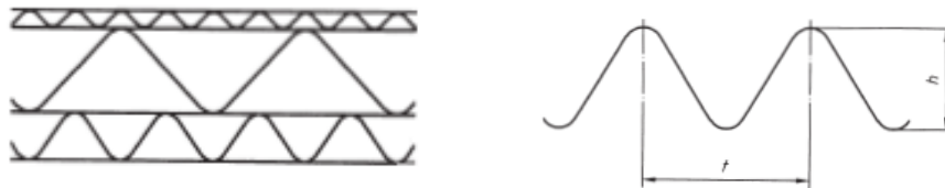
Figure 8.2-1: Triple-wall corrugated fiberboard (left) and Flute dimension (right)
